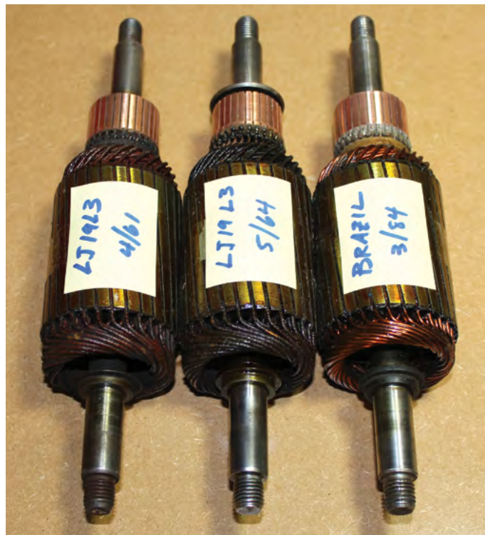
Figure 3: Three tested, cleaned, and machined Bosch 6V armatures made in Germany and Brazil from 1961 to 1984.
