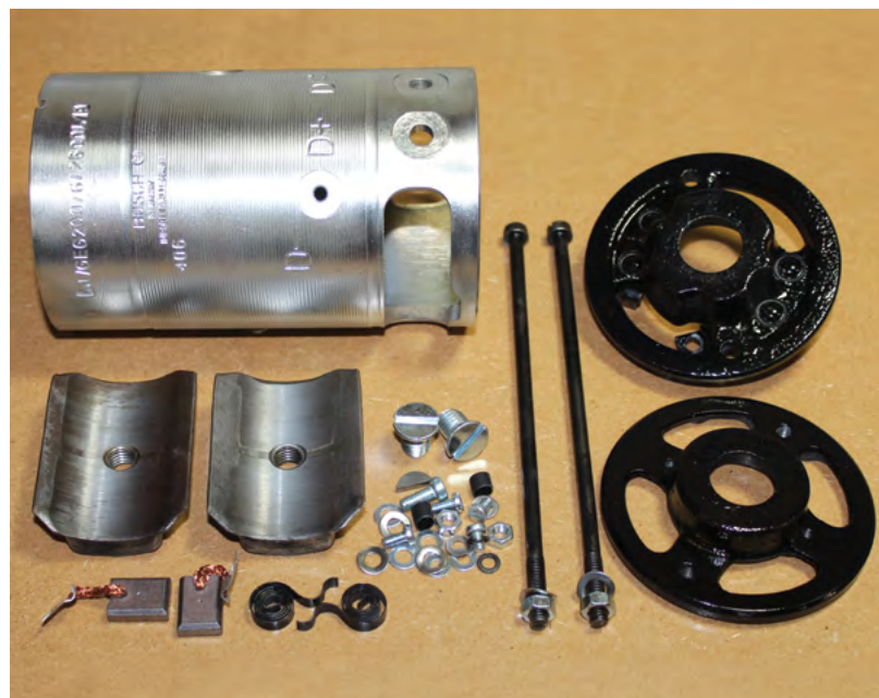
Figure 6: The zinc-plated generator housing, painted end caps, new pole shoe screws, new brushes, pole shoes, springs, and hardware.
