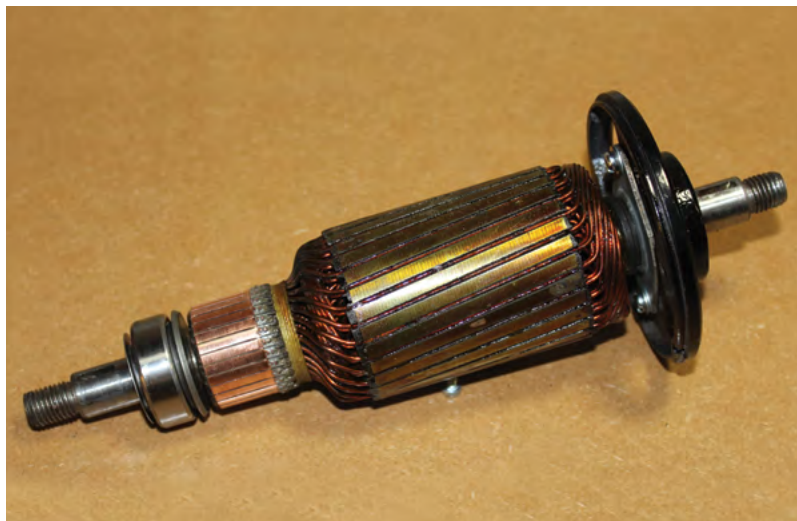
Figure 8: The fully assembled armature with the end cap, ready to insert into the housing.
