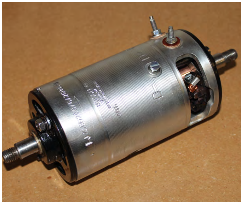
Figure 9: The completed generator, ready to install.
