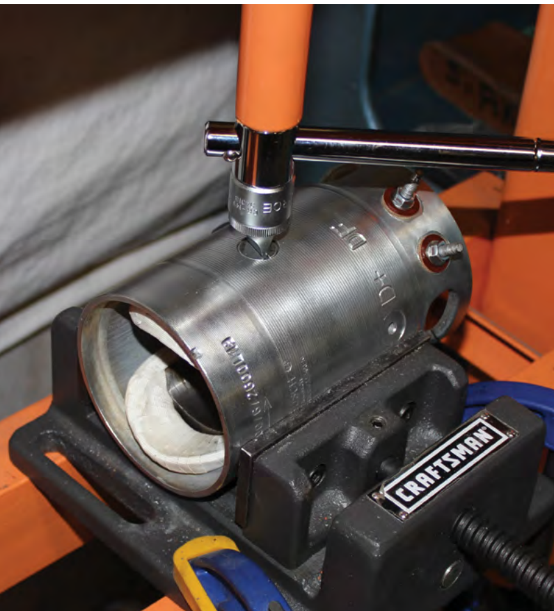
Figure 7: A shop press with a breaker bar and a 1/2-inch drag socket is used to get the torque needed to tighten the two pole screws.
