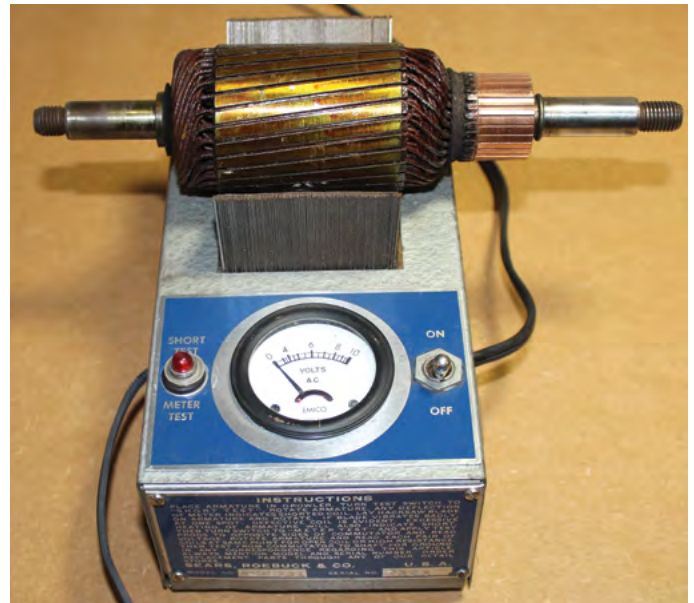
Figure 1: Armature testing for shorts, opens, and grounds is done using a growler.
