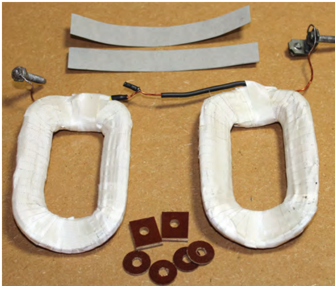
Figure 5: Re-soldered and re-wrapped field coils with high-temperature shrink tubing, together with new phenolic and fish paper insulators.
