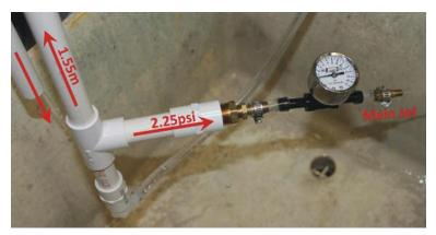
A 1.55 meter water column constructed to measure the flow rate though main jets. Water flows through the bottom of the column, up 1.55 meters past the 'head' to a vented u-fitting and drains off and down. The jet under test is at the end of the head and receives water at the constant relative pressure of 2.25 psi.
