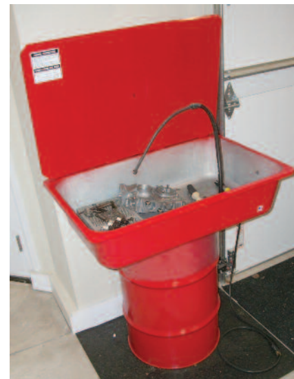
A drum style washer capable of larger solvent volumes and parts. This 30 gallon system is from TP tools and is similar to those sold by Safety Kleen and others.
