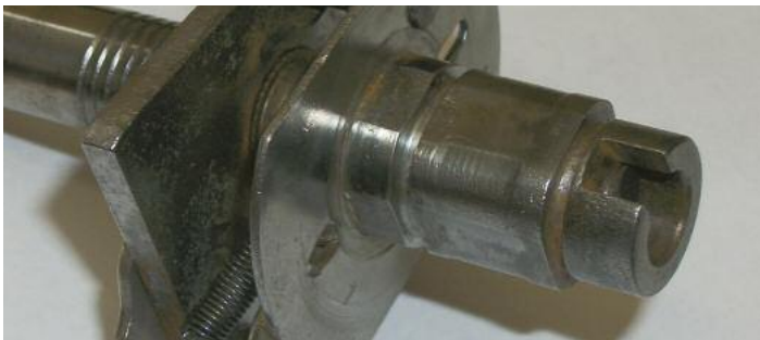
A heavily worn cam on a 50+ year old distributor leading to variation between the lobes.
