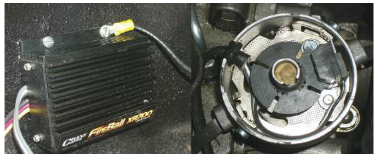
A Fireball XR700 installed in a 912 with the ignition module on the firewall (left) and optical sensor in the distributor (right).
