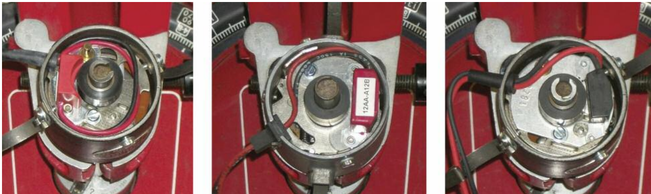
Electronic ignition modules installed in distributors: the Hot Spark in a 022 distributor (left), the Ignitor II in a 050 distributor (center), and the Ignitor I in a BR18 distributor (right).
