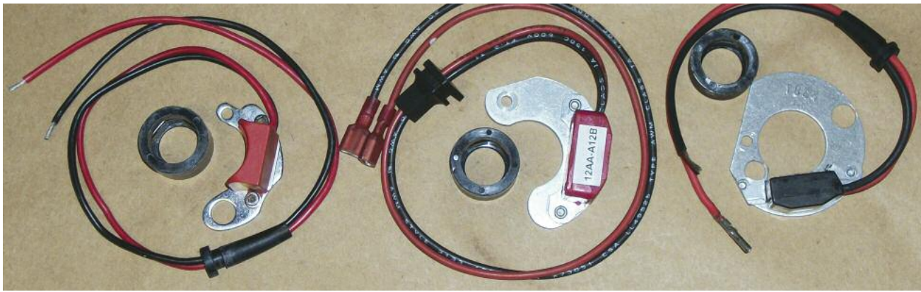
Three Hall-effect electronic ignition modules: Hot Spark (left), Pertronix Ignitor II (center), and Pertronix Ignitor I (right).
