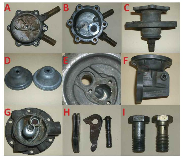
valves aren't usually physically damaged. Instead they may be harmed by a heavy residue buildup. Once the pump top is clean, you can test the valve action by gently blowing/sucking the output fuel line or the input section at the top cavity. If you get a mouthful of something, I didn't tell you to do it.
