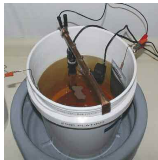
The zinc electroplating tank using a five gallon bucket. Anodes are on either side of the parts which are suspended with wire from the top plating bar.
