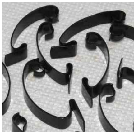
Bosch distributor clips, an example of items with a phosphated finish
