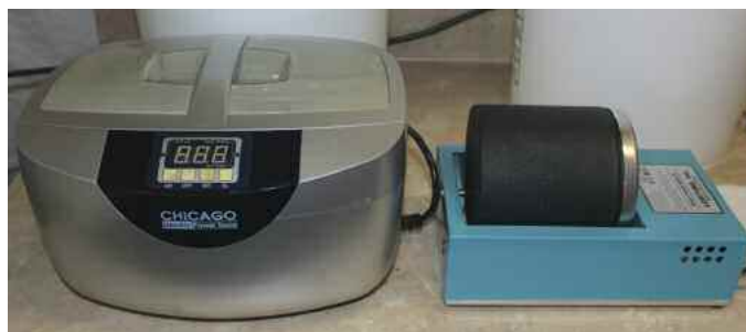
A small ultrasonic cleaner (left) and a rotary tumbler (right) for parts cleaning. Vibrating tumblers are also available.
