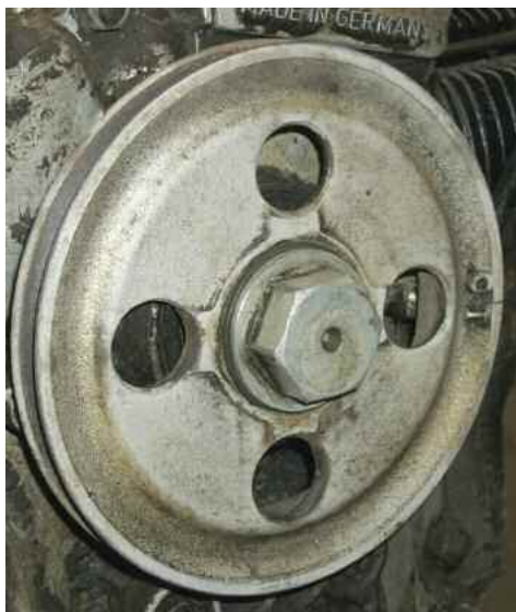
A generator pulley, spring washer and pulley bolt with unique protective coatings. The difference in appearance between the bolt and pulley are from roughness of the underlying parts.
